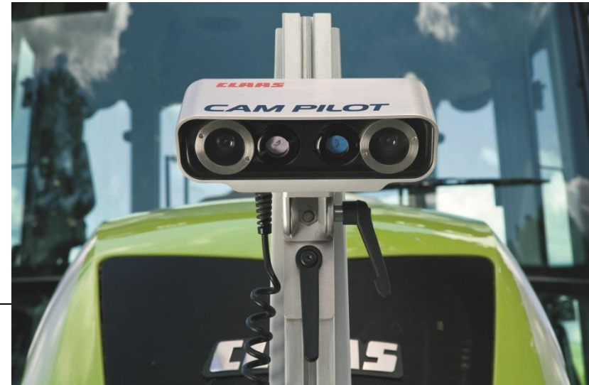
Claas Cam Pilot – 3D-Kamera
